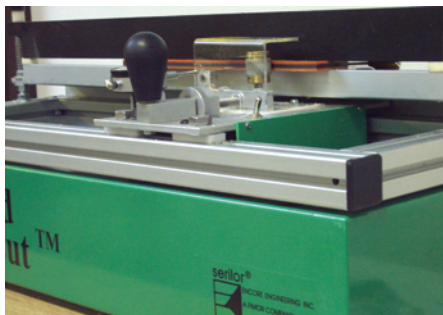
Figure 1: Diamond wheel squeegee grinder (Fimor).
